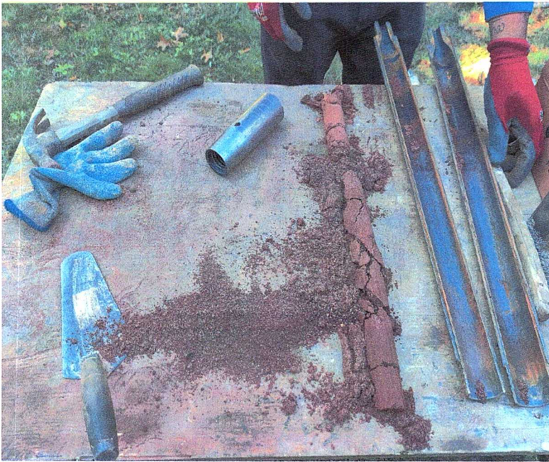
Sample recovery from split spoon samplers
