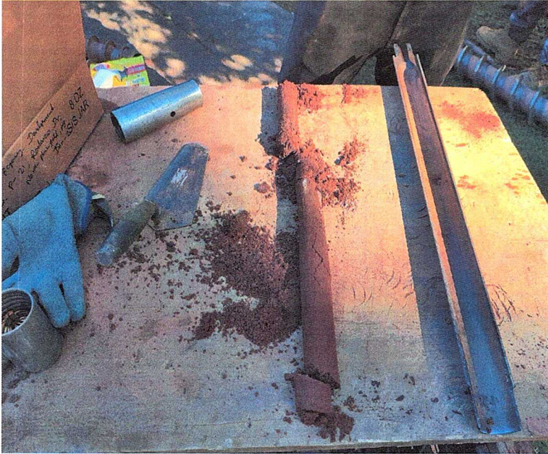
Sample recovery from split spoon samplers
